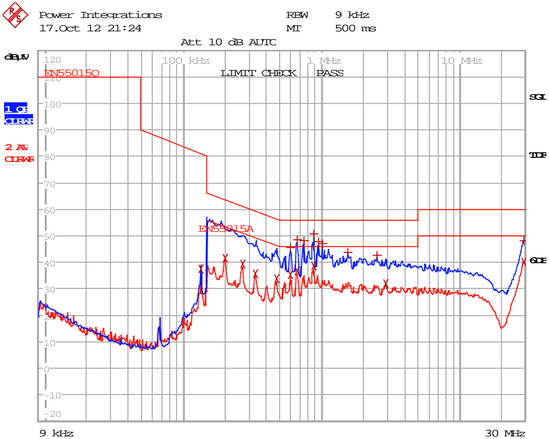
Figure 27 – Conducted EMI, Maximum Steady State Load, 230 VAC, 60 Hz, and EN55015 B Limits.
