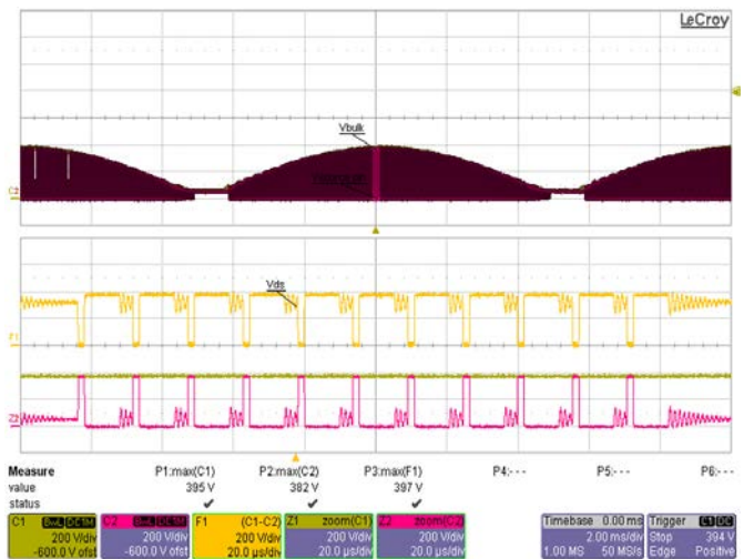
Figure 19 – 265 VAC, Full Load F1(Orange): V_{DRAIN-SOURCE} , 200 V / div. Ch1(Yellow): V_{DRAIN-GND} , 200 V / div. Ch2(Red): V_{SOURCE-GND} , 200 V, 2 ms / div. Z1(Yellow): V_{DRAIN-GND} , 200V / div. Z2(Red): V_{SOURCE-GND} , 200 V, 20 \mu s / div.
