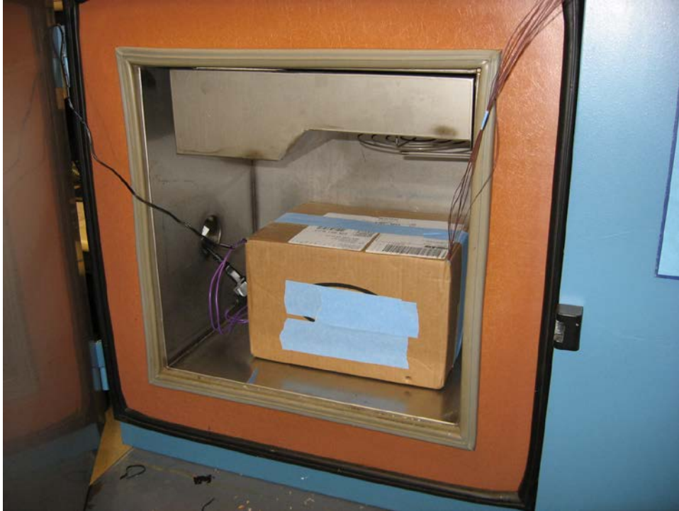
Figure 11 – Thermal Chamber Set-up Showing Box Used to Prevent Airflow Over UUT.
