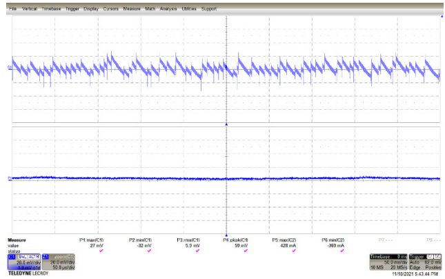
Figure 61 – Output Voltage Ripple. V_{IN} = 500 \text{ VDC} , I_{OUT} = 0 \text{ A} . Upper: V_{OUT} , 20 mV, 50 ms / div. Lower: Zoom @ 50 \mu\text{s} / div. V_{RIPPLE} = 99 \text{ mV}_{P-P} .
