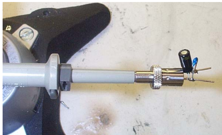
Figure 27 – Oscilloscope Probe with Probe Master 5125BA BNC Adapter. (Modified with wires for probe ground for ripple measurement, and two parallel decoupling capacitors added)
