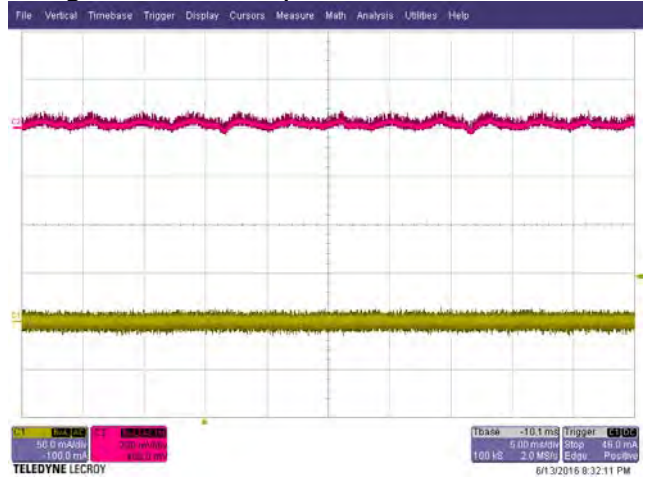
Figure 33 – Output Voltage and Current Ripple in CV Mode, 230 VAC, Chroma CC Load, 2.8 A Setting. Upper: Output V_{RIPPLE} , 200 mV / div. Lower: I_{OUT} Ripple, 50 mA, 5 ms / div.
