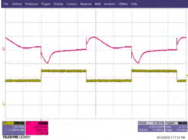
Figure 28 – Output Transient Response, CV Mode, 50%-75%-50% Load Step, 115VAC 115 VAC Input. Upper: V_{OUT} , 200 mV / div. Lower: Main Output I_{LOAD} , 1 A, 2 ms / div.
