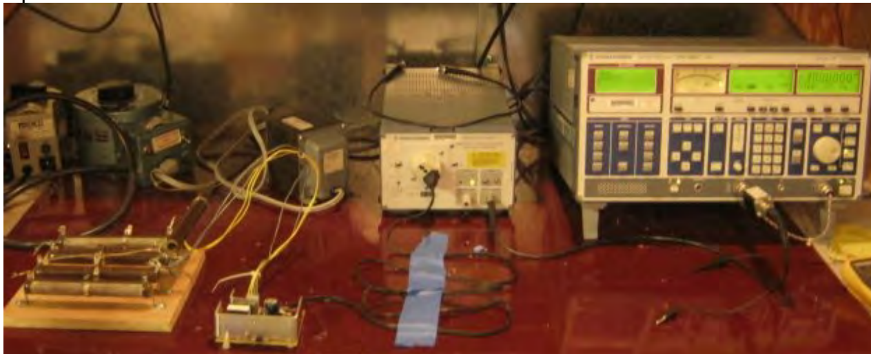
Figure 42 – EMI Set-up with Floating Resistive Load.
