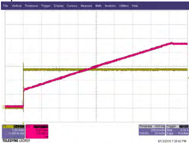
Figure 22 – Output Start-up, Constant Voltage Mode, 115 VAC, Chroma CC Load, 2.8 A Setting. Upper: V_{OUT} , 5 V / div. Lower: I_{OUT} , 1 A, 200 ms / div.
