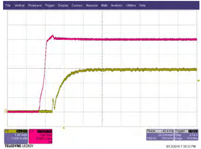
Figure 27 – Output Start-up, Constant Current Mode. 230 VAC, Chroma CV Load, 10 V Setting. Upper: Main V_{OUT} , 2 V / div. Lower: Main I_{OUT} 1 A, 20 ms / div.
