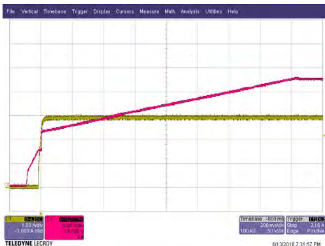
Figure 24 – Output Start-up, Constant Current Mode, 115 VAC, Chroma CV Load, 22 V Setting. Upper: Main V_{OUT} , 5 V / div. Lower: Main I_{OUT} , 1A, 200 ms / div.
