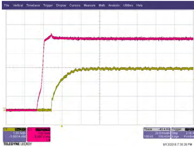
Figure 26 – Output Start-up, Constant Current Mode, 115 VAC, Chroma CV Load, 10 V Setting. Upper: Main V_{OUT} , 2 V / div. Lower: Main I_{OUT} , 1 A, 20 ms / div.
