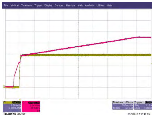
Figure 25 – Output Start-up, Constant Current Mode. 230 VAC, Chroma CV Load, 22 V Setting. Upper: Main V_{OUT} , 5 V / div. Lower: Main V_{OUT} 1 A, 200 ms / div.
