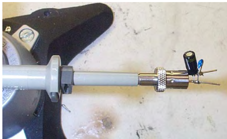
Figure 31 – Oscilloscope Probe with Probe Master 4987BA BNC Adapter (Modified with Wires for Probe Ground for Ripple measurement and Two Parallel Decoupling Capacitors Added).
