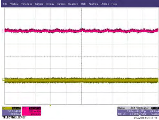
Figure 32 – Main Output Voltage Ripple, 115 VAC, CV Mode, Using Chroma CC Load, 2.8 A Setting. Upper: Output V_{RIPPLE} , 200 mV / div. Lower: I_{OUT} Ripple, 50 mA, 5 ms / div.
