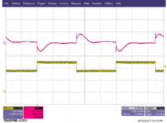
Figure 29 – Output Transient Response, CV Mode, 50%-75%-50% Load Step, 230 VAC Input. Upper: V_{OUT} , 200 mV / div. Lower: Main Output I_{LOAD} , 1 A, 2 ms / div.
