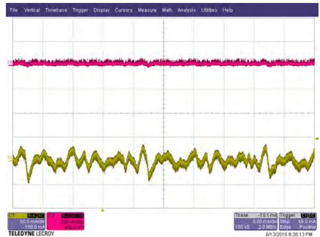
Figure 35 – Main Output Voltage and Current Ripple in Constant Current Mode, 230 VAC, Chroma CV Load, 22 V Setting. Upper: Main Output V_{RIPPLE} , 200 mV / div. Lower: I_{OUT} Ripple, 50 mA, 5 ms /div.
