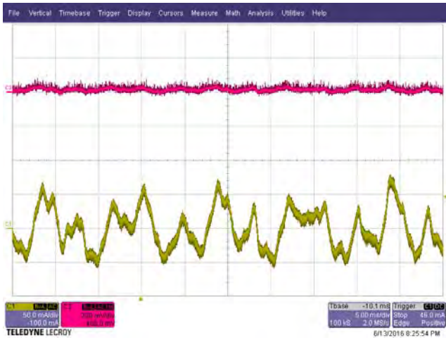
Figure 36 – Main Output Voltage and Current Ripple in Constant Current Mode, 115 VAC, Chroma CV Load, 10 V Setting. Upper: Main Output V_{RIPPLE} , 200 mV / div. Lower: I_{OUT} Ripple, 50 mA, 5 ms /div.
