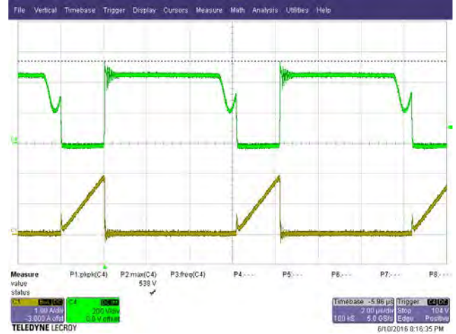
Figure 19 – Primary Voltage and Current, 230 VAC Input, 100% Load. Upper: V_{DRAIN} , 200 V / div. Lower: I_{DRAIN} , 1 A / , 2 \mu s / div.
